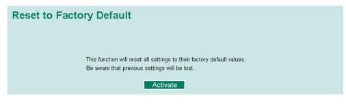
The Factory Default function is included to give users a quick way of restoring the EDS's configuration settings to their factory default values. This function can be accessed from either the telnet/RS-232 Console, or Web Browser interface.
